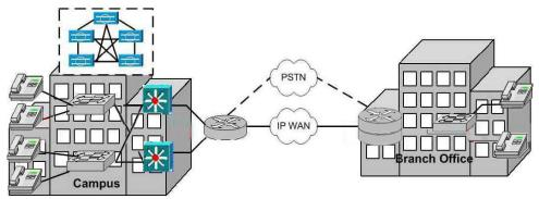
Given the network shown in the exhibit, select the recommended QoS configuration for the slow speed WAN segment connecting the campus and branch office.
