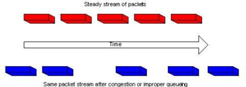
When a router receives a Real-Time Protocol (RTP) audio stream for Voice over IP (VoIP), it must compensate for the jitter that is encountered. The mechanism that handles this function is the playout delay buffer. The playout delay buffer must buffer these packets and then play them out in a steady stream to the digital signal processors (DSPs) to be converted back to an analog audio stream. The playout delay buffer is also sometimes referred to as the de-jitter buffer.
