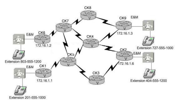
In the VoIP network above, which protocol provides the necessary sequence numbers so voice packets originating at CK1 are played in the correct order to CK5?
